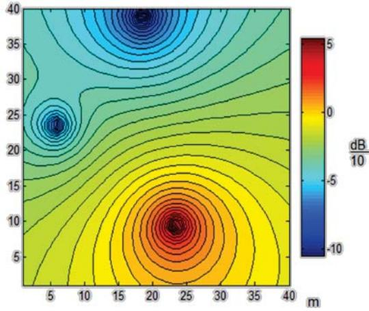
Fig. 1: A SIR coverage map of the target of the bottom transmitter.
