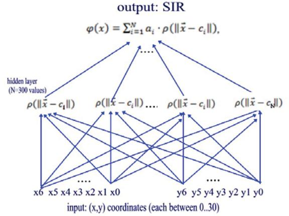
Fig. 2. The radial basis network used for the task of SIR learning, with  $N$
