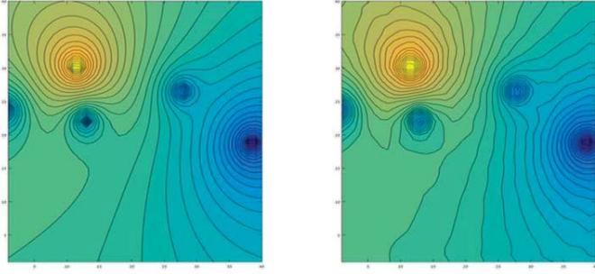
Fig. 4. left: A typical randomly created coverage map for 5 transmitters (4 interferers). Right: the coverage map learned by the RBN.
