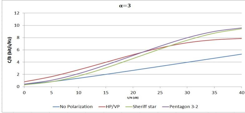
Fig. 8 Spectral efficiency in a pentagon -  $\alpha = 3$ .
