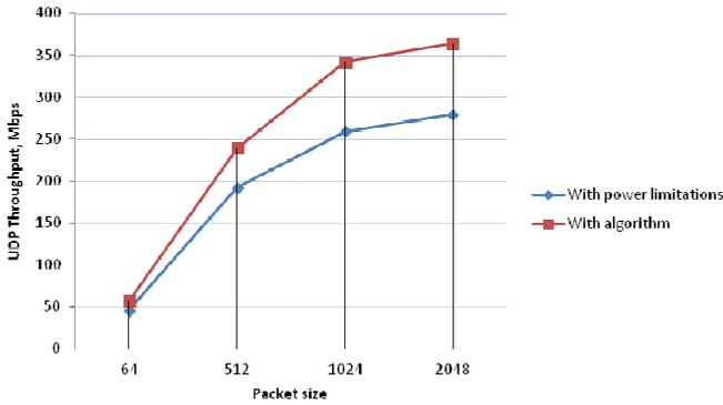
Fig. 5. Total throughput in a given Wi-Fi channel, as a sum of throughputs of all devices using that channel
