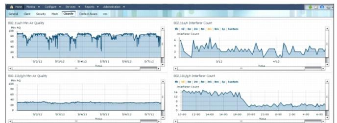
Fig. 2. Monitoring various spectrum parameters in the Cisco CleanAIR Prime Network Control System [43]
